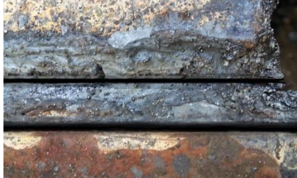
3/16" and 3/8" cuts using a .375" Exoblade™
