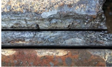
3/16" and 3/8" cuts using a .375" Exoblade™
